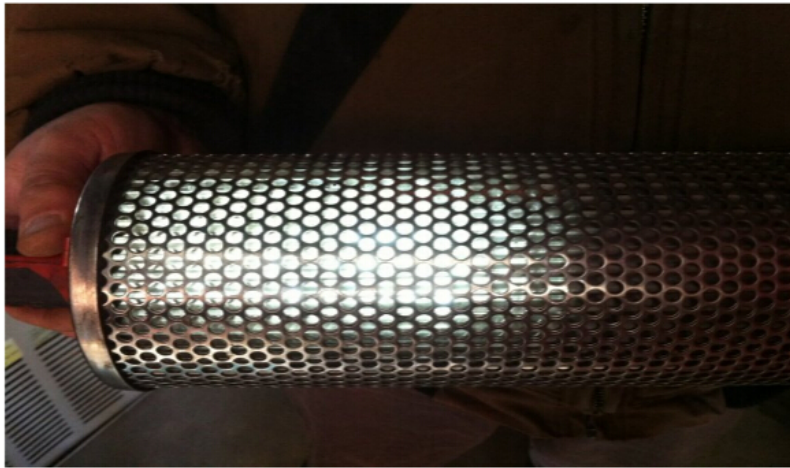
Cleaned oil filters with Light passing through
